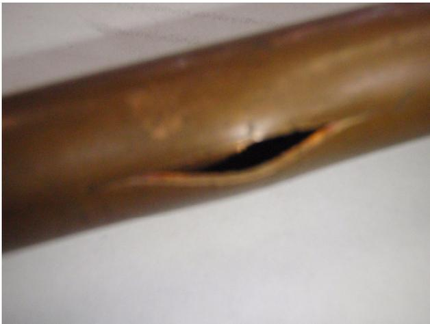
This pipe was exposed to single digit temperatures and burst within 20 minutes of exposure. Water damage doesn't always occur when the pipe splits, but, rather when the pipe thaws out. Many times people think that they are out of the danger of bursting pipes after a cold night, however, it may be a few days later when the flooding occurs.
